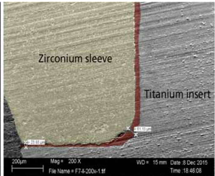
Fig. 2: Magnification of the external bonding gap (L1) with a size of 0.21 μm. The gap of the bonding joint is therefore more than half as small as for adhesive mounting of crowns on teeth, where a bonding joint of 50 μm is regarded as being ideal.
