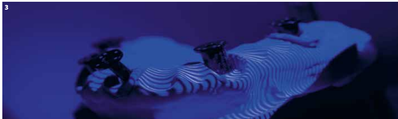
Figure 3: All parts of the model relevant to our work are scanned using structured blue LED light.
