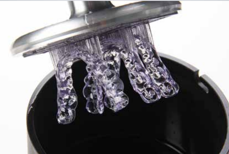
10 - 13 The printed splint is removed and carefully detached. The fit on the model is unprecedented. After a final polymerization in the light-curing unit (on the model), the splint is ready for insertion. The entire procedure was comprised of only a few steps
