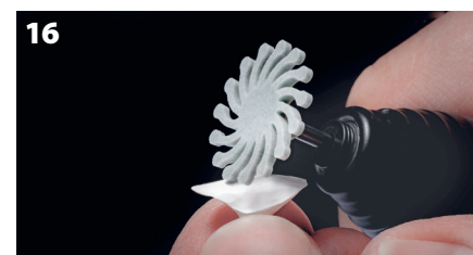
Fig. 16: Careful preparation is already a central process step in the unsintered green state (Panther, Sirius ceramics). Novel instruments work in a material-friendly, efficient manner and leave no unwanted residues on the material's surface.
