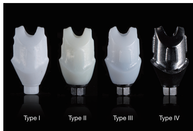
Fig. 2. Samples of the investigated CAD-CAM abutment types I-IV from left to right. Type I: zirconia monotype abutment (CADAbut F, BeCe CAD Zirconia XH), type II: lithium disilicate hybrid abutment (CADAbut D, IPS e.max CAD LT on Ti-Base), type III: zirconia hybrid abutment (CADAbut D, Zirconia LT CAD on Ti-Base), type IV: titanium monotype abutment (CADAbut F, CAD Titanium).
